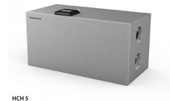
The HCH 5 residential ventilation unit is primarily designed for 1-2 family houses. The unit is supplied as packaged ventilation units complete with built-in demand-control and a control panel. The residential ventilation units are fitted with highly efficient counterflow heat exchangers which are optimised to a very high efficiency level thus achieving a very low specific fan power (SPI value) for the entire unit.
