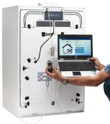
CALIBRATION VIA PC TOOL
